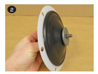
Apply a couple drops of a medium strength thread locker, such as Loctite® 246, to the outer plate bolt (item 19). Thread the shaft (item 27) onto the bolt until it is snug to the flat back side of the inner plate (item 22).
