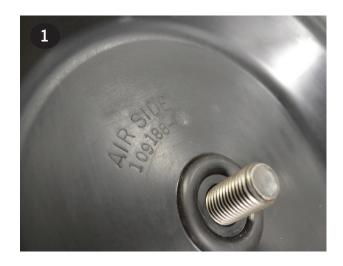
Place the inner plate (item 22) over the bolt. Ensure the round recess in the plate faces the diaphragm (item 21).
