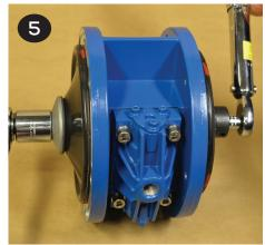
Remove the outer plate, diaphragm(s), and inner plate (items 18, 20/21 & 22) from the side that is loosened. Pull or push the shaft (item 27) and remaining plates and diaphragms out of the center section. If pulling, it may be easier to grip the diaphragm if it is inverted.
